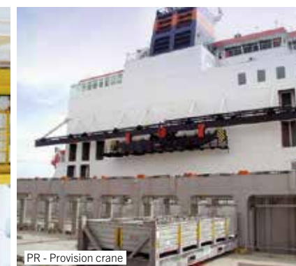
PR - Provision crane
