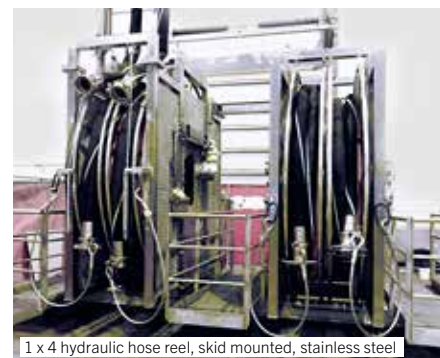
1 x 4 hydraulic hose reel, skid mounted, stainless steel
