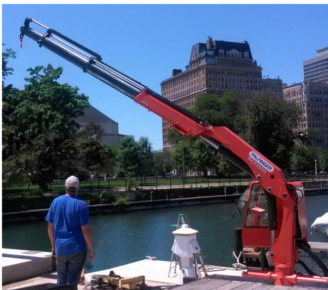
Picture: Barge mounted PK 23500 (M) B freshwater helps now to manage the harbor system in the Chicago Park District.
